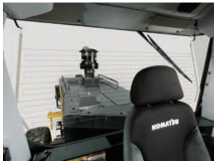
The low and narrow engine hood offers a clear view to the rear
